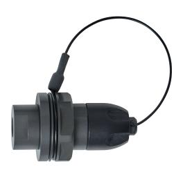
The FALCON connectors offer the best attenuation values and smallest 12-channel connector foot print on the market. With an insertion loss of <1,2 dB it outperformes NATO specification (<2,5 dB). This is achieved with Micropol's lens technology, state of the art production and alignment process.
