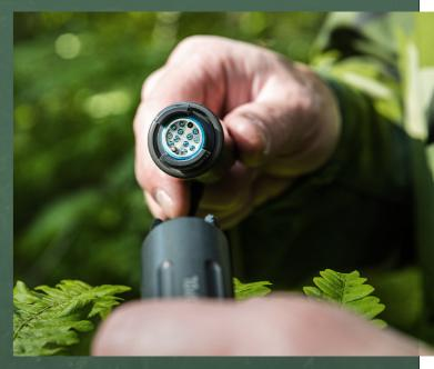
OptiScan measures the signal strength of optical fiber lengths, providing quick confirmation of link attenuation to secure optimum function. Field measurements are easy to carry out and deliver fast, reliable results
