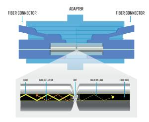
Inspecting BOTH sides of the fiber connection is the ONLY WAY to ensure that wil be free of contamination and defects
