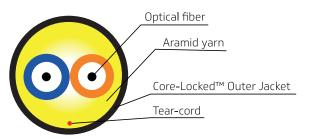
The HD tactical cable is ideal for usage in harsh environments, developed to be used where size and weight are important factors for transport and usage.
